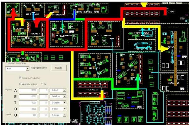
Figure 1: Flow Path Calculator – used as a static material flow optimization tool
